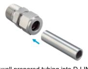
1. Insert well prepared tubing into D-LINE two ferrule tube fittingsuntil tubing end is firmly seated on the body shoulder.
